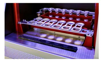
The revolutionary adaptive burner control system allows the user to set the burner temperature electronically at the user interface. The ABCS then automatically modifies flow parameters to ensure this temperature is achieved and maintained throughout the fusion cycle.
